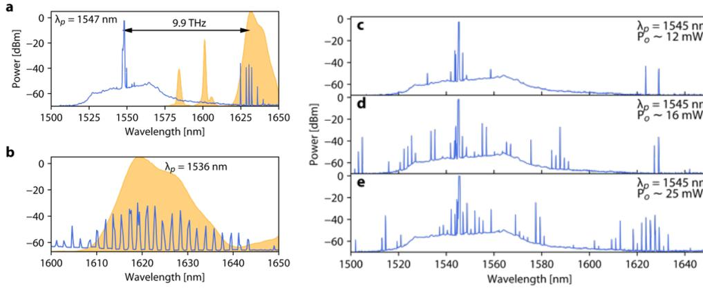
Fig. 2. Experimental observations of Raman lasing and Kerr combs in a hybrid MR. (a) Few lines Raman comb when pumping near 1547 nm. (b) Raman comb when pumping a high-Q resonance near 1536 nm. The shaded curves in (a) and (b) show the Raman response spectrum of bulk  $\text{As}_{20}\text{S}_{80}$ . (c),(d),(e) Co-existence of Raman comb and Kerr combs components when pumping near 1545 nm at on-chip pump power of 12 mW, 16 mW and 25 mW, respectively.
